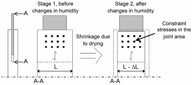
Figure 5 Constraint stresses caused by the moisture-induced deformations being restrained by the dowels, which are fixed in position by the steel plate.
