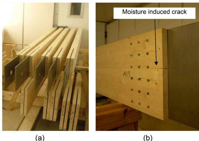
*Figure 9 (a) Storage of joint-specimens in climate chambers (observe that for the specimens below the dowels and the plate are not fitted yet) and (b) a moisture induced crack in a joint-specimen exposed only to drying*
