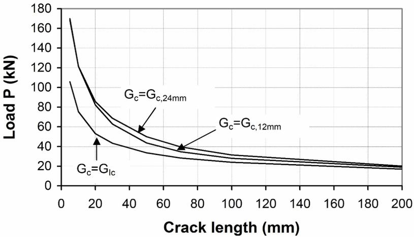
Figure 15 Relation between crack load, initial crack length and various choices of  $G_c$  of an inverted double-tapered glulam beam. Calculations are based on the energy release rate approach.
