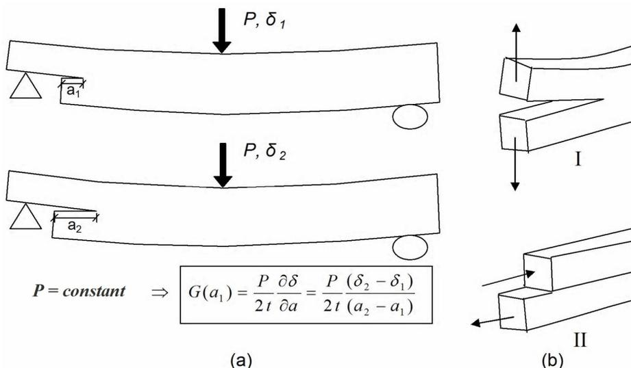
Figure 14 (a) An example of how to calculate the energy release rate  $G$  of a notched glulam beam and (b) definition of the modes of loading and fracture relevant for this work.
