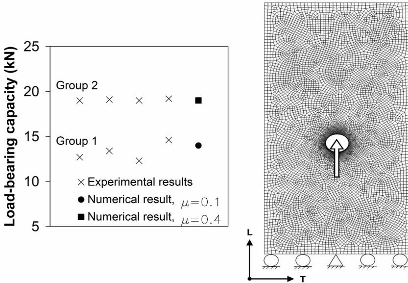
Figure 17 Load-bearing capacity of single dowel joints. Numerical and experimental results for different dowel surfaces. For group 1, the dowels had a smooth surface and for group 2, the dowels had a rough surface.
