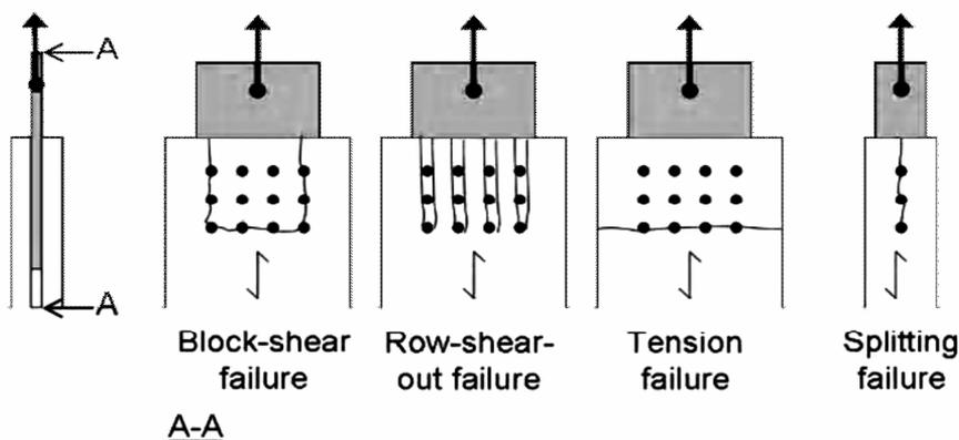
Figure 4 Expected final failure modes for multiple dowel joints loaded in tension parallel to the grain.
