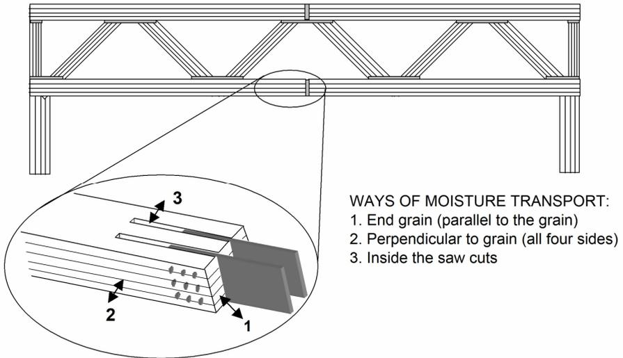
Figure 6 Ways of moisture transport in a steel-timber dowel joint.
