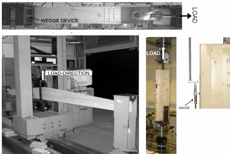
Figure 10 Loading-arrangement for the specimens.
