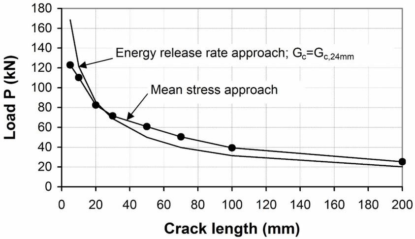
Figure 16 Relation between crack load and initial crack length of an inverted double-tapered glulam beam. Calculations are based on the energy release rate approach and the mean stress approach.
