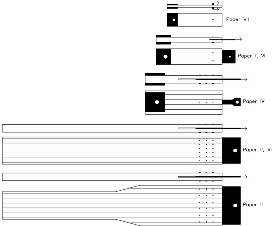
*Figure 7 All joint specimens tested. The different geometric setups are drawn to scale in proportion to each other.*
