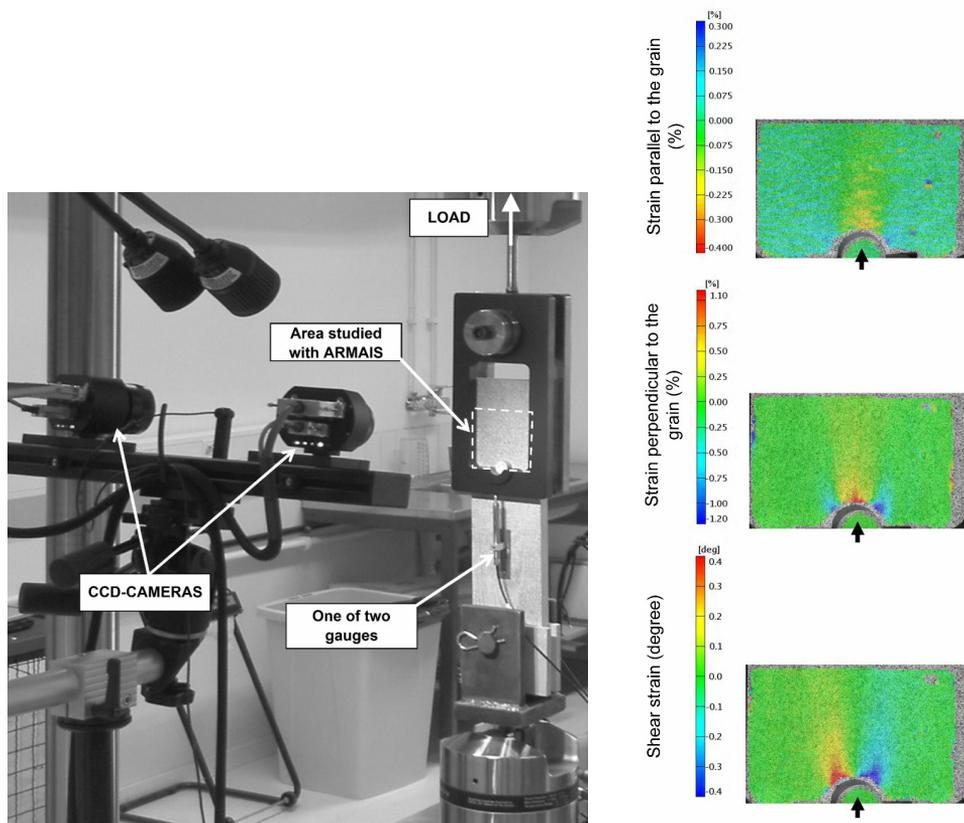
Figure 12 Contact-free measurement arrangements in Paper VII and some results.
