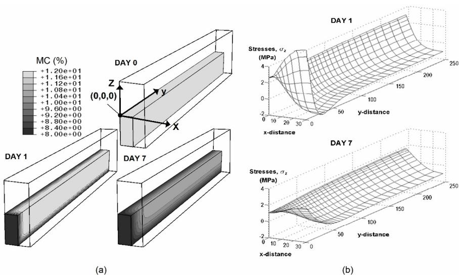
Figure 13 Result from Paper III: Changes in MC of a glulam beam (60·150·700 mm<sup>3</sup>) during drying from 65% RH to 20% RH and belonging stresses perpendicular to the grain presented on the symmetry surface.
